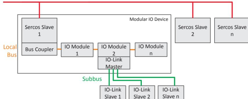
Image 2: Modular device with an integrated gateway
