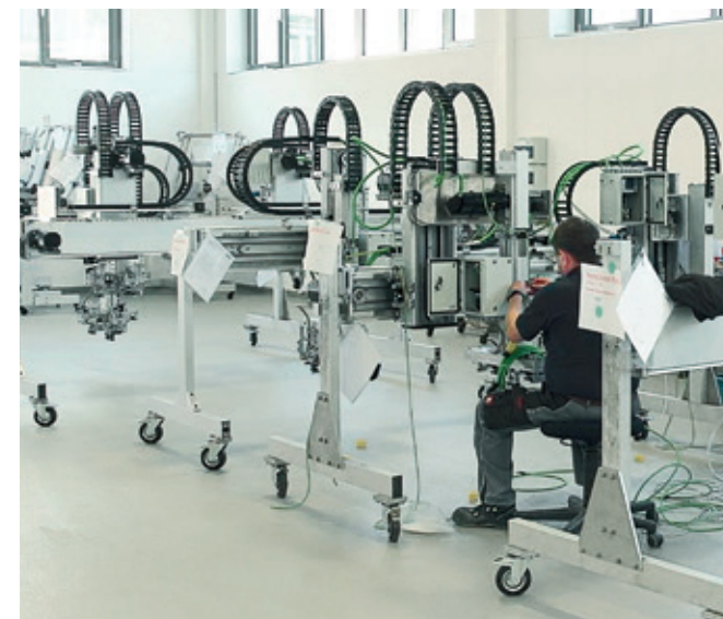
Image 1: Mechatronic modules with complete modular servo drive technology on rollable assembly and transport frames
