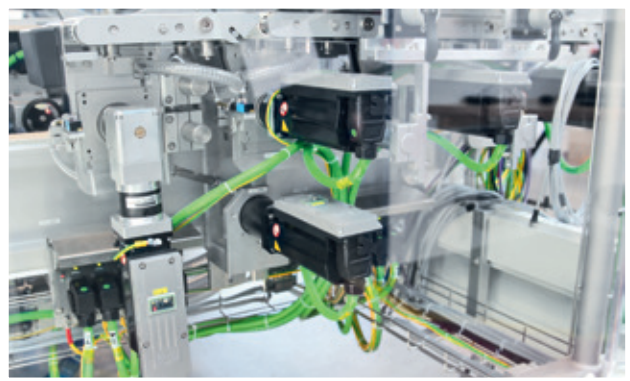
Image 4: The drive electronics for the Lexium 62 ILM piggyback on each servomotor, saving space in the control cabinet.
