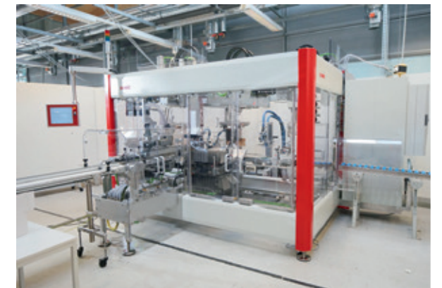
Image 2: Modular end-of-line packaging machine: Functionality is enhanced through customized configuration of mechatronic units within the machine frame.
