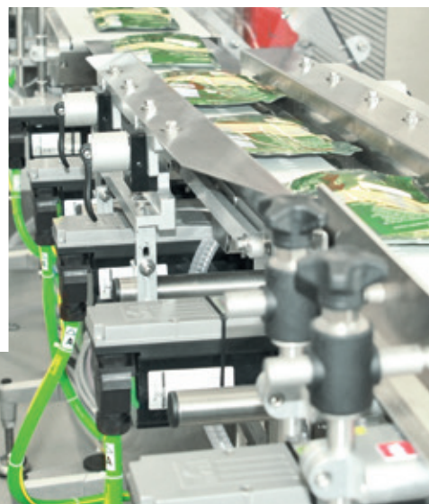
Image 5: Innovative approach: Conveyor system with servo technology instead of asynchronous motors controlled by variable frequency drives: full integration into the motion control unit's communication and software solution, engineering advantages, and much greater flexibility offset higher product costs on the purchasing side.
