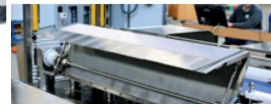
*"Bridging the gap": The bridge, which is unfolded by a servo motor, reduces space requirements in the isolator.*
