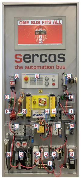
**B** The **Bosch Rexroth** IndraControl VAM 10/40 machine control panel features 2x15 short-stroke buttons and programmable LED indicators. Feedrate and spindle speed override switches can be scaled in software. E-stop and power ON/OFF pushbuttons can be wired into the machine's power circuit. www.boschrexroth.com/controls.
