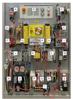
N The **LinMot** C1250 servo drive with the Sercos automation bus offers 32-bit position resolution and an integrated power stage, ideal for standard and high-end positioning tasks with NC-synchronization in the low voltage range, 24-72VDC. LinMot linear motors employ a direct electromagnetic principle. Electromagnetic force provides direct linear movement without the use of cams, gears, belts, or other mechanical devices. www.linmot.com
