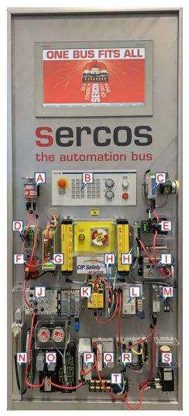
R The Bosch Rexroth IndraControl S67 IO system enables reliable, cabinet-free installation near the machine, even in harsh environments. A wide range of digital and analog I/O, temperature, communication and function modules with fast performance is available. Built in diagnostics for supply voltage, overload and communication is available on Sercos. Standard M12 and M8 connections ensure quick and secure connections to peripherals.
