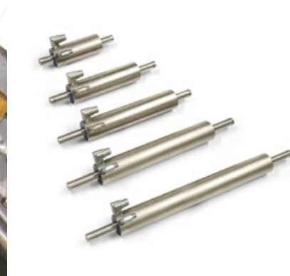
Figure 5: The linear motors in the P10-70 series are the most powerful motors in the LinMot catalog, with peak forces of up to 2,500 N. Thanks to their modular design, their strokes can range between 10 and 1,770 mm.
