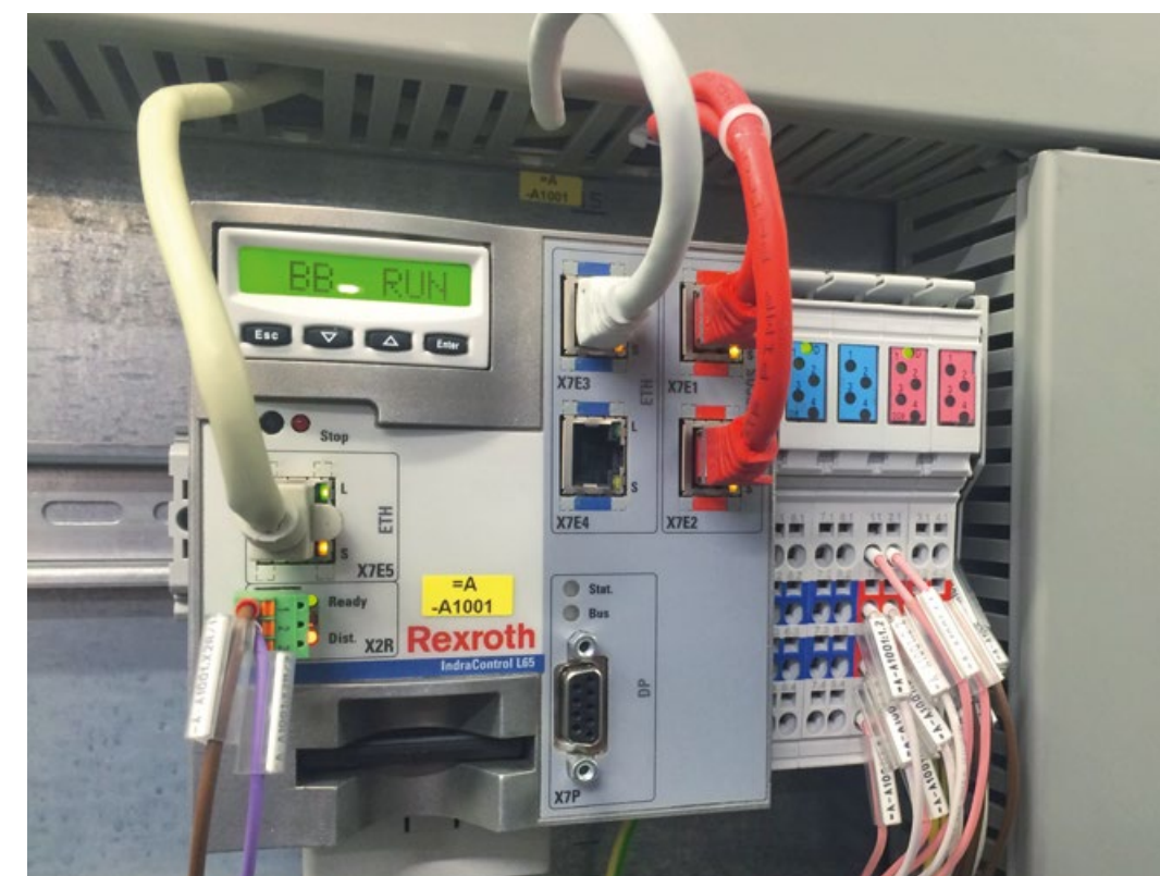
Figure 7: A controller from Bosch Rexroth (IndraControl L65) handles the coordination of the numerous axes on the new molding machine, as well as calculating the motion profiles of the LinMot linear motors. This allows Chocolat Frey to react rapidly and flexibly to new product requirements.
