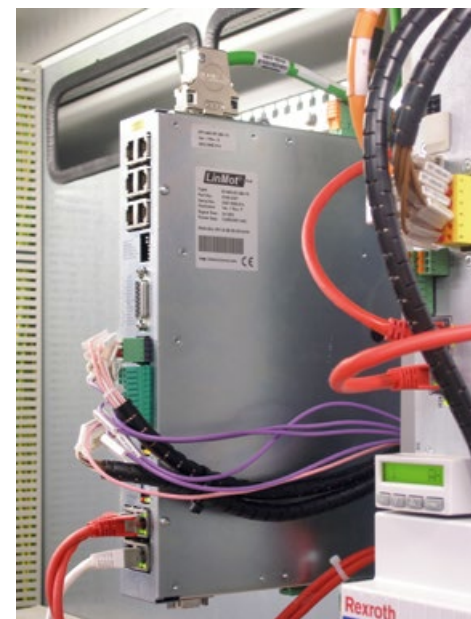
Figure 6: The E1400 controller with direct feed supplies the P10-70 linear motor with sufficient power. Various interfaces, such as Sercos III (shown here), Profinet, or Powerlink are available for connecting to the motion control system.
