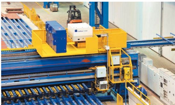
Efficient technology – The laser welding system from Firma Held Systems Deutschland used for building ships at the Meyer Werft in Papenburg. Controlled with CNC from IBH Automation, Kornwestheim.
