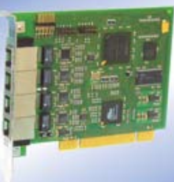
FPGA-based, active or passive PCI module
