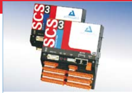
SCS 3 – a compact and modular control and IO system with SERCOS III master or slave interface
