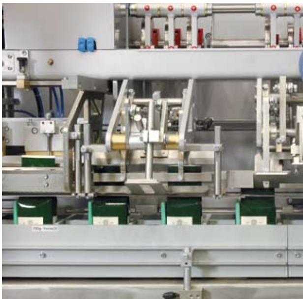
Two bags are filled and closed in parallel (picture shows the multi-stage folding and closing process)
