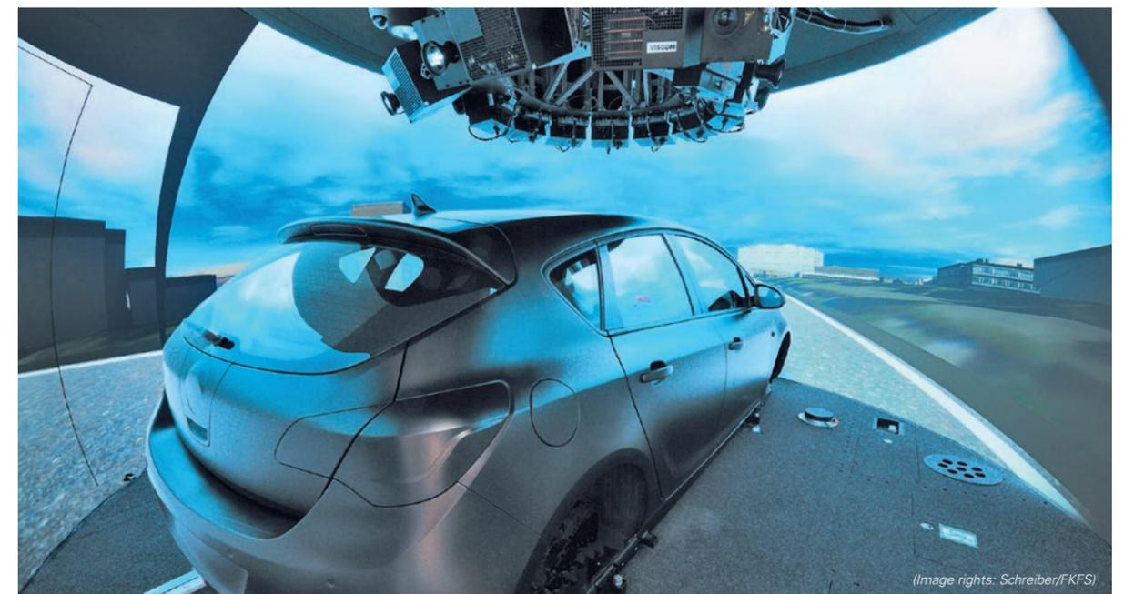
In the dome: The projectors can be seen above the vehicle.
