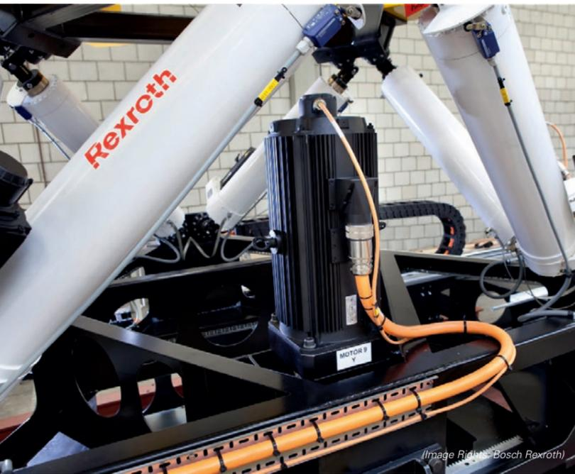
AC servomotors move the hexapod over the gantry system in the Y direction
