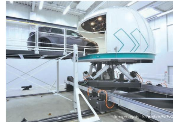
Europe's largest driving simulator is housed at the University of Stuttgart and can handle a payload of 4,000 kg. This allows tests with a complete vehicle.
