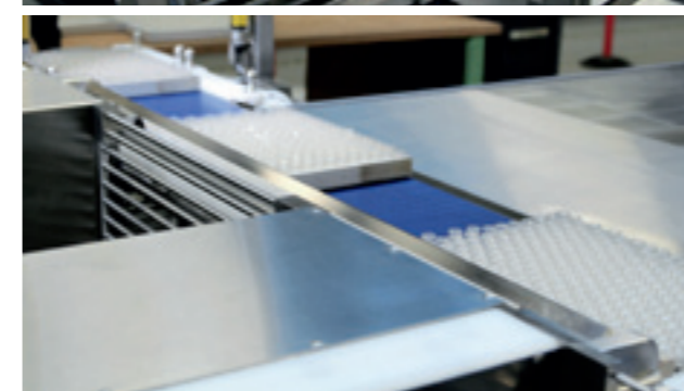
The vials, shown here on optional tablets, approach the unit and are then pushed across the bridge by a slide into the freeze dryer. The process is reversed after the freeze drying process is complete.
