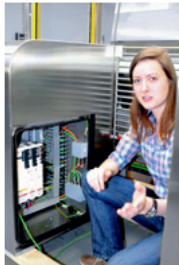
Anne Gerlach, ALUS Development/GEA Lyophil, explains the structure of the PacDrive automation solution with shared power supply.
