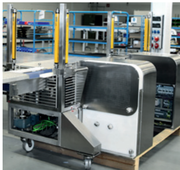
A new mobile ALUSTM unit in the assembly/test phase: On the left, the buffer table with conveyor belt; below, outside of the hygiene-critical area, the integrated Lexium ILM62 drives with cabling.
