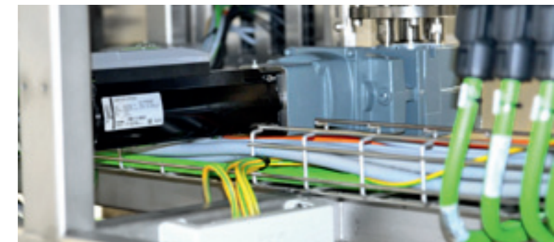
The Lexium 62 ILM servo drives, connected with the distribution boxes and hybrid cables, are located in the base of the ALUS, outside of the hygiene-critical area.
