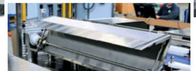
"Bridging the gap": The bridge, which is unfolded by a servo motor, reduces space requirements in the isolator.
