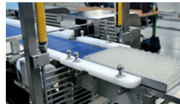
"Bridging the gap": The bridge, which is unfolded by a servo motor, reduces space requirements in the isolator.
