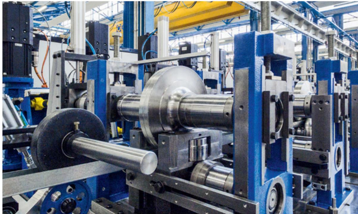
The new production line, 65 m long and 6 m wide, able to work from 2 to 40 m of sheet metal per minute and produce metal profiles with a 500 mm development, measuring 300 x 100 mm and 5 mm thick, is now ready to leave the new plant in Mirano (in the province of Venice) and be installed at the premises of the customer – a German firm specializing in the subcontracting of profiling and requiring a system with exceptional production versatility features.
