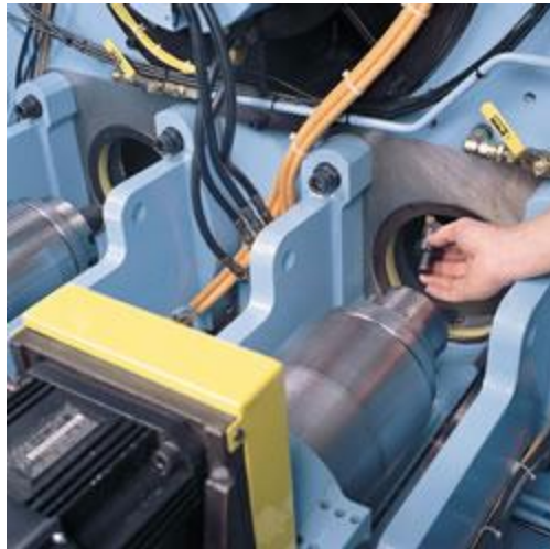
Quick and easy tool change via sliding spindle carrier.
