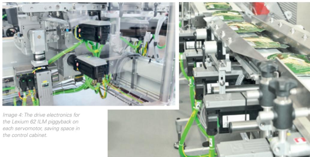
Image 4: The drive electronics for the Lexium 62 ILM piggyback on each servomotor, saving space in the control cabinet.
