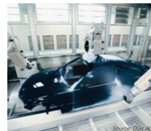
Figure 1: Exact spray head positioning and pressure control by means of synchronous communication
