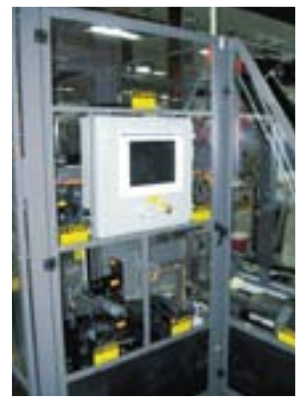
Mounted on the machine frame, the Rexroth IndraControl VEP40 HMI uses a Windows CE-based platform and integrates easily with the rest of the control system.
