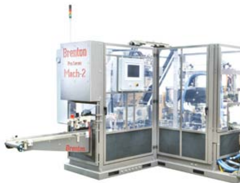
The Brenton ProSeries Mach-2 uses a Rexroth motor integrated drive and motion logic control platform to improve machine performance, save space, lower costs and save energy.
